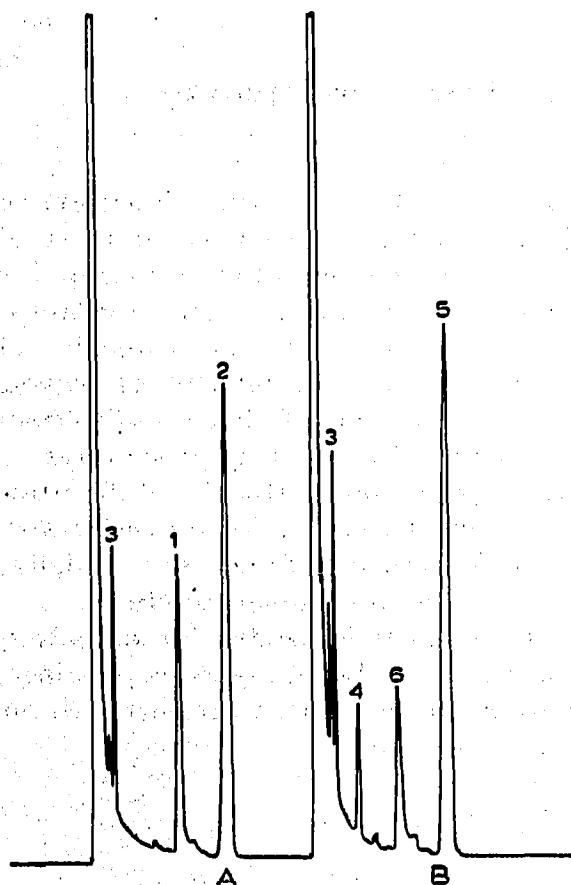
Fig. 3. Comparison of serum (patient) sample with recovery of 3 mg % dilantin. A, 3 mg % recovery; B, unknown serum sample. Peaks: 1, recovery of 3 mg % dilantin in acetone; 2, decyl stearate (internal standard); 3, phenobarbital; 4, unknown; 5, decyl stearate; 6, dilantin.
